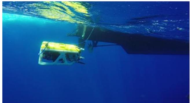
*The Remote Operate Vehicle (ROV) is used to evaluate the status of the benthic areas surveyed during the field surveys carried out in the 3 involved countries.*
